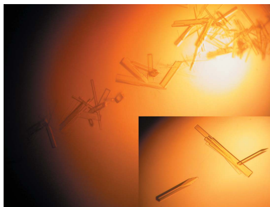
Figure 4 Picture of a typical \Delta^4 -(5 \alpha )-KSTD crystallization drop. The crystals grew in a line through the drop as a consequence of the streak-seeding procedure. The inset shows a close-up of the crystals. Single crystals with approximate dimensions of 500 × 100 × 100 \mu m were used for data collection.
